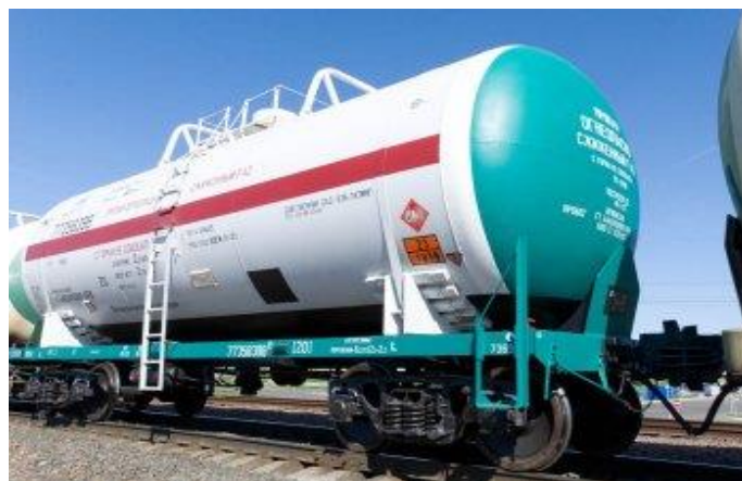
Figure 1. Wagon-tank for liquefied gas transportation.
